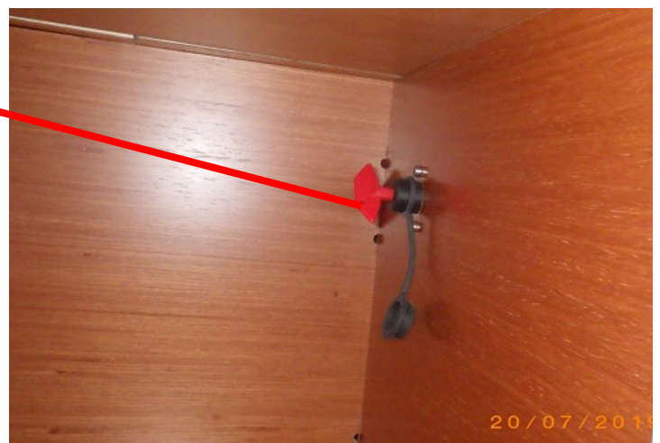
Fuse and switch of bowthruster located in space under the bed of bow cabin.
