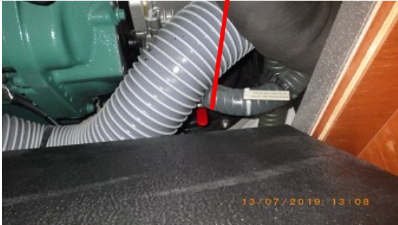
Engine cooling water inlet
