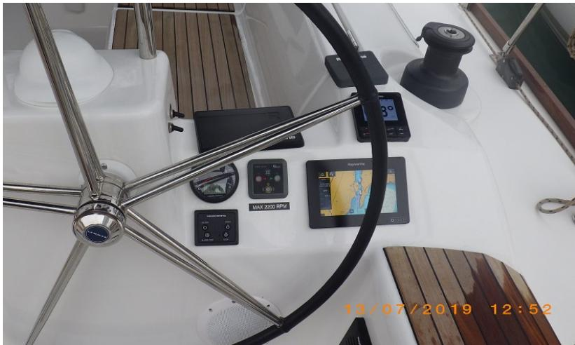
Raymarin i70 multifunction instrument (<http://www.raymarine.com/display/?id=17721>), and compass located at the port side helm.
