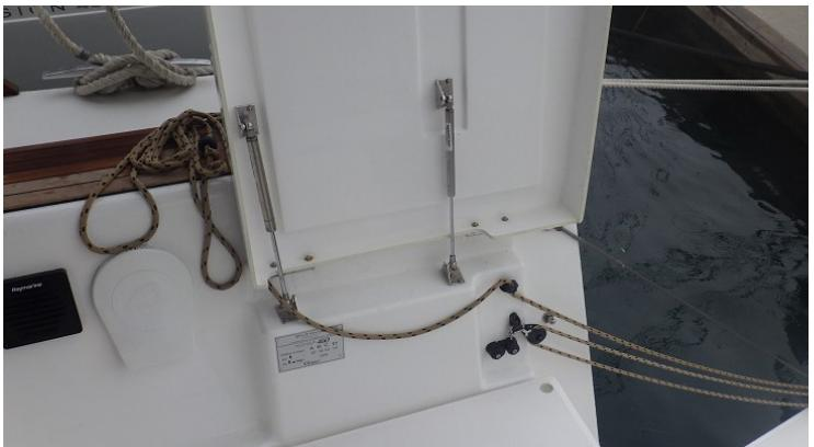
Yacht is equipped with retractable transom (bathing platform). There is a swim ladder. While under sail, the transom should remain closed and secure. After you have gotten to your anchorage feel free to deploy the transom for easy access to your dinghy, swimming or snorkeling.
