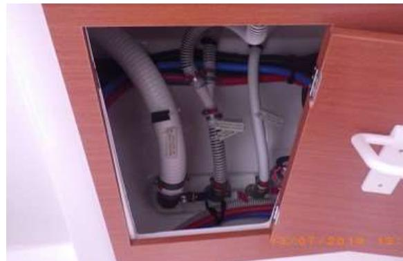
**Valve handle to switch waste tank located under the floor plate between bow heads.**
