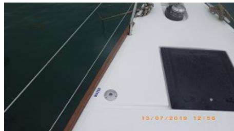
Unscrew the plug using a winch handle. A fresh water level indicator is located on the electrical control panel. The tanks are connected, so that the water level is equal in all tanks when both valves are open.
