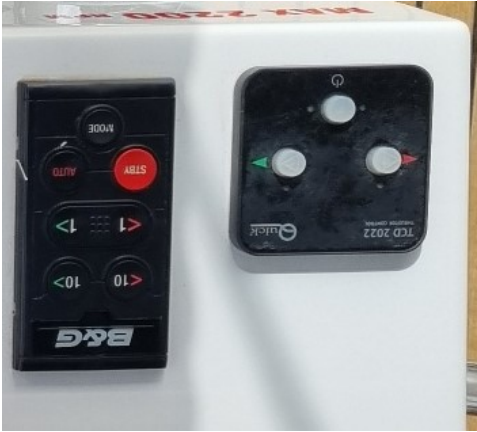
Remote control of bowthruster Quick (maximum time of continuous operation 5 seconds).
