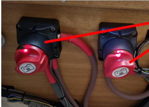
Main switch for Servis batteries Starter battery Anchor windlass
