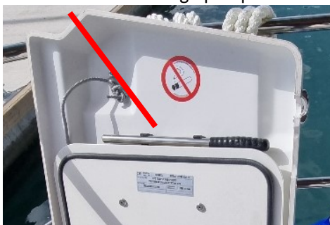
Manual bilge pump on port side skipper helm seats. Handle for manual bilge pump.
