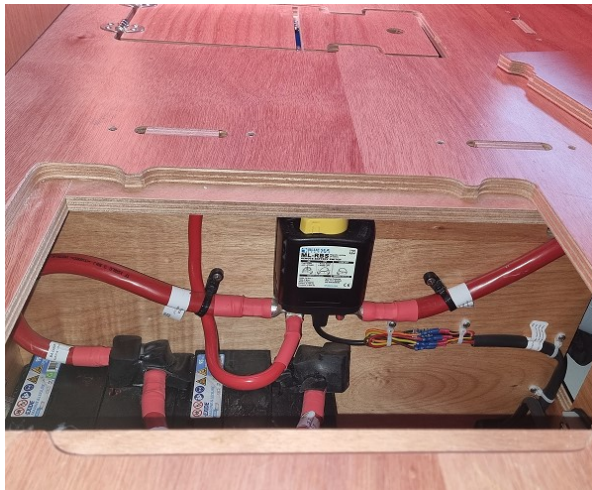
Bow thruster battery switch is under the bow cabin bed.
