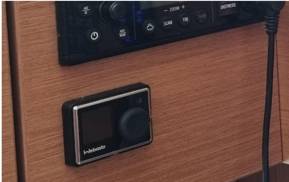
Turn off the heating by pressing the top button on the remote control.
