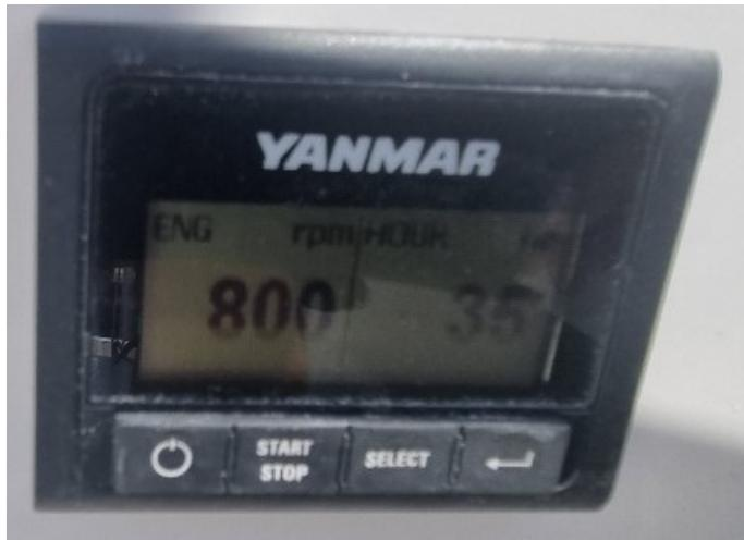
**Should you hear an engine alarm during operation, check the screen to identify the reason for the alarm (over heating/oil pressure/battery) immediately shut down the engine-CALL Technical support.**
