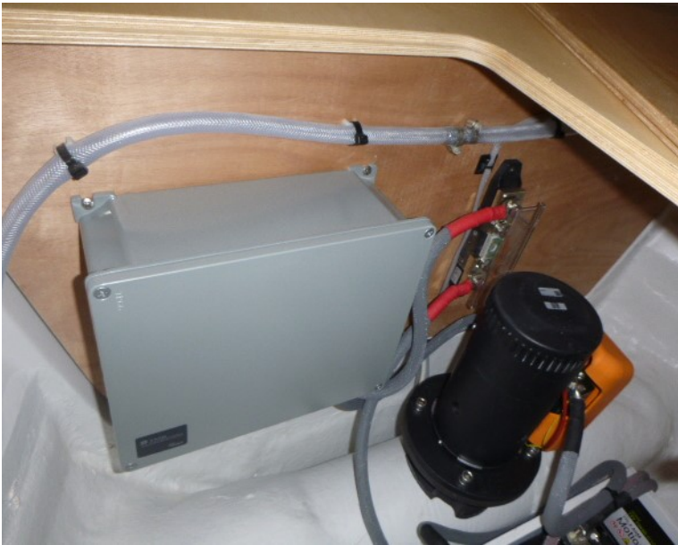
Remote control of bowthruster Quick (maximum time of continuous operation 5 seconds).
